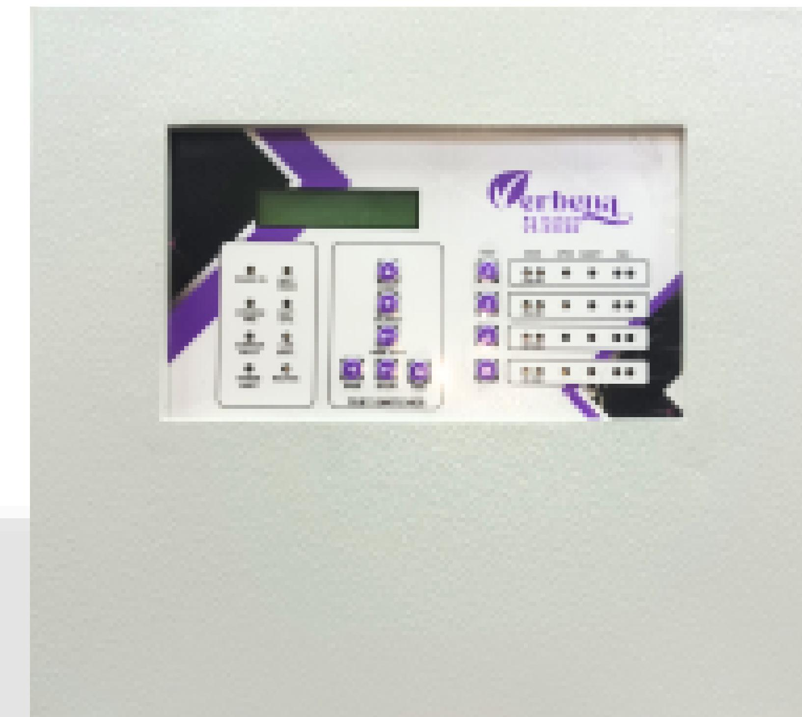
In case of an events of fire and fault, It will indicate the respective zone on its console and also perform the required function like activating the hooters of the respective zone. Each Zone can have a maximum of 20 Conventional Detectors. Panels are featured to integrate with auto dialler and third-party systems with potential free contact.
