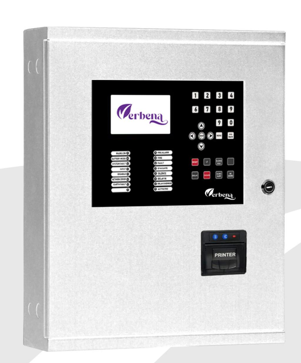
Logging capacity of 7000 Events. Multiple levels of password protection facility, Complete Front panel Programmable /Software configurable Fire Alarm Control Panel. MODBUS connectivity (Optional). Panel to panel networking support up to 1kms. Cause and Effect matrix across 64 panels in Networking. Shall be IOT compatible with Verbena Range of Conventional Panels in Single Mobile Application
